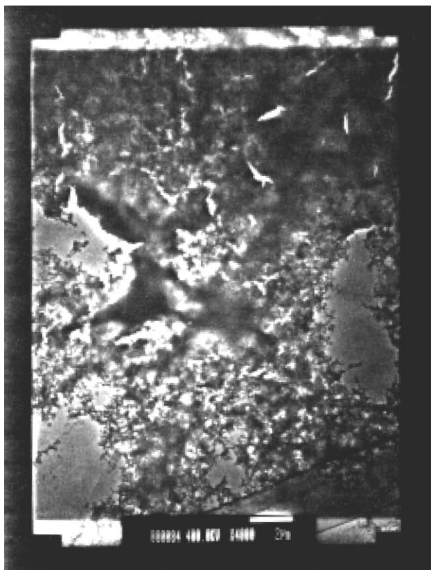
Fig. 1. Electron micrograph of the precipitated ladder polymer on a copper grid.
